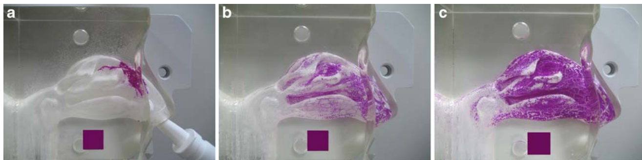
Fig. 5. Deposition patterns of Normal saline in Afrin spray bottle (a), Pari Sinustar (2 min) (b) and Pari Sinustar (5 min) (c).
